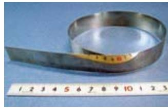
図 2  $\text{Ni}_3(\text{Si},\text{Ti})$  冷間圧延板
